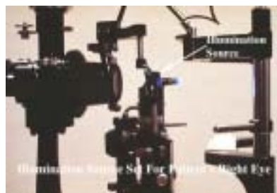
Correct Illumination Source Placement. Temporal to the Tonometry Probe for patient's right eye.
